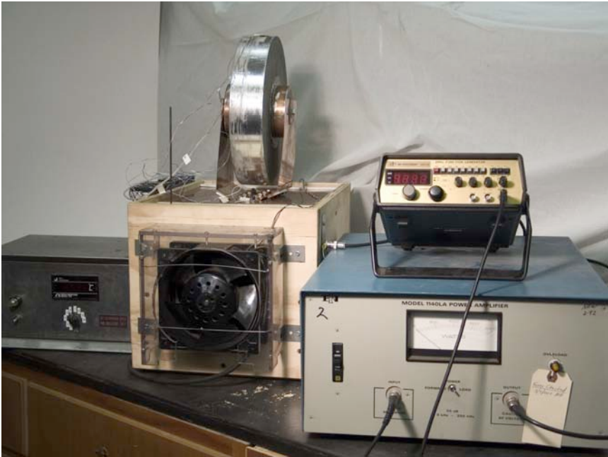
Figure 6. Photograph of the ripple current test stand
