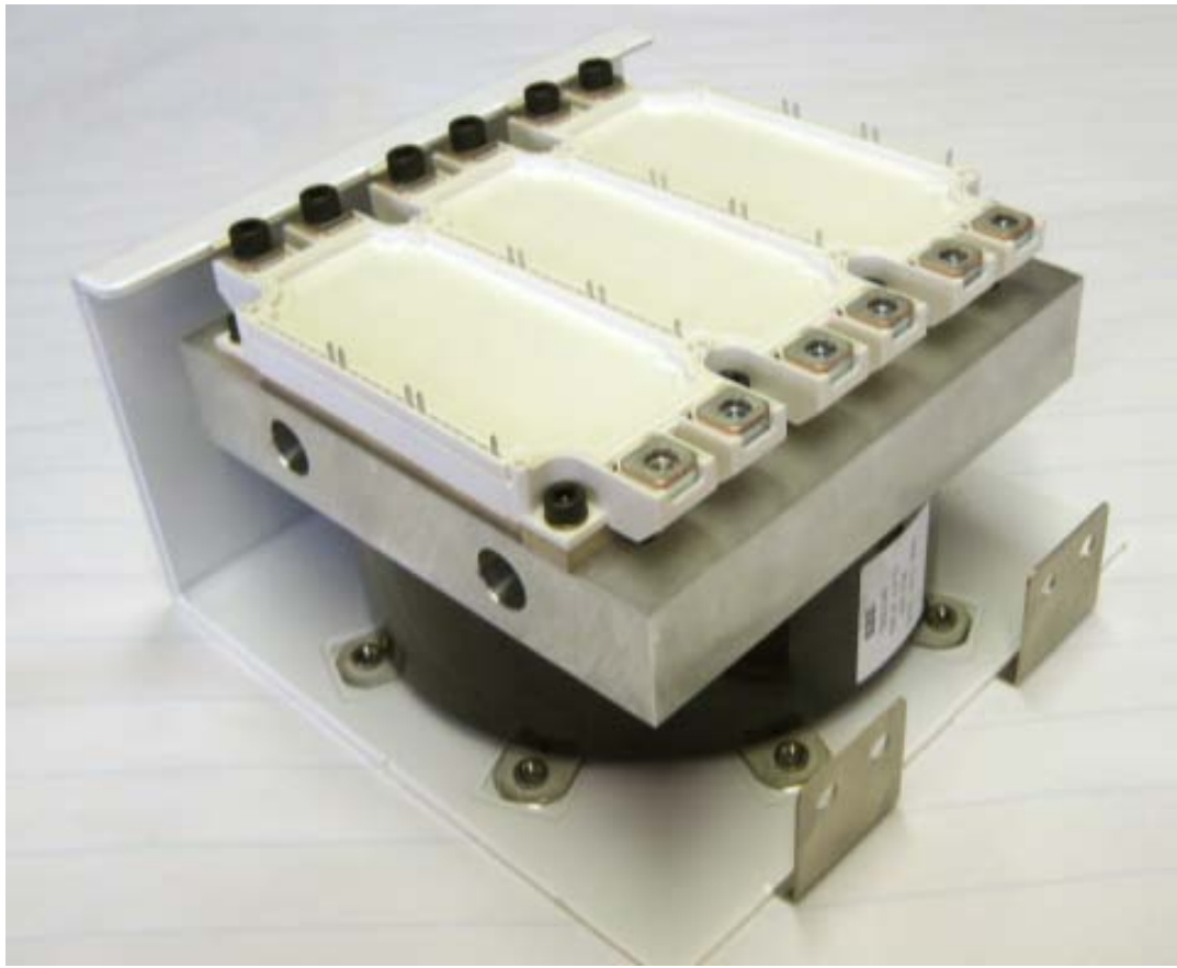
Figure 3. Vertical inverter configuration capacitor and bus.
