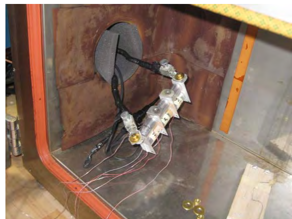
Figure 3. Three stage capacitor array installed in climate chamber prior to testing
