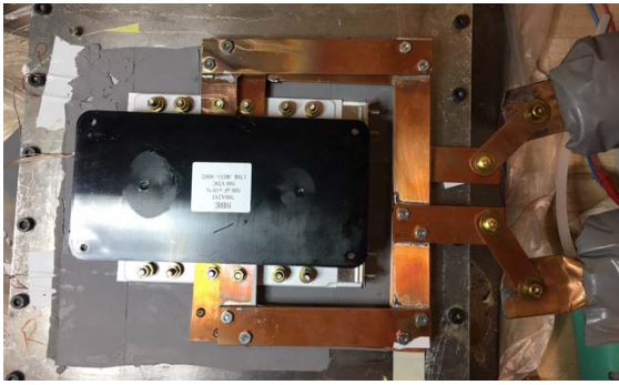
Fig. 3. SBE 700A243 500µF 500V integrated capacitor/bus installed on cooling plate and connected to ripple current source for temperature rise testing.
