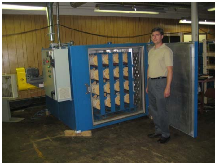
Fig.2. Photograph of capacitor specimens and mounting rack for a single thermal chamber.
