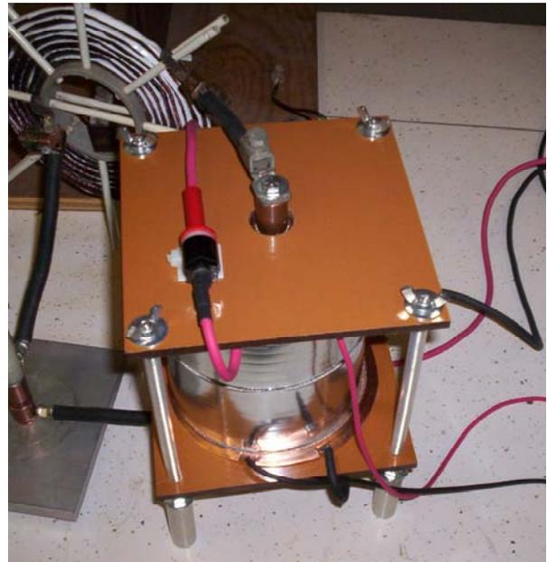
**Figure 2.** Photograph of the series capacitor stack.
