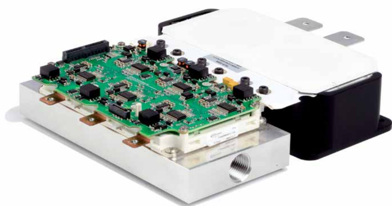
Figure 1: Integrated capacitor/bus DC link from SBE Inc.
