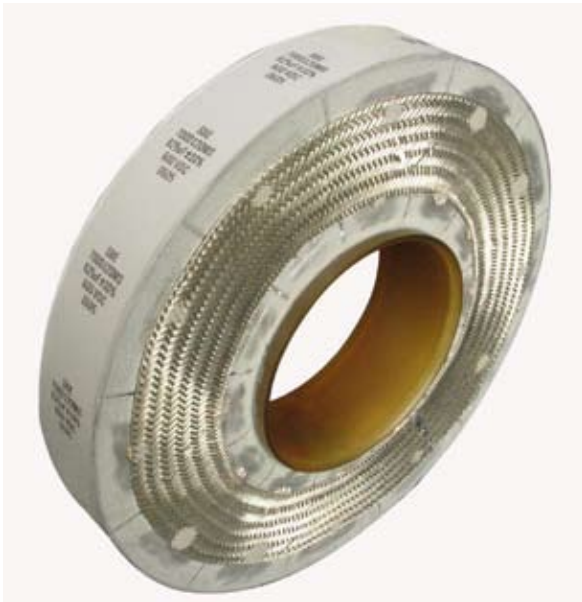
Figure 3: Photo of the new innovative annular ring geometry capacitor using metalized polymer film with a center hole area sufficient for inverter semiconductor population
