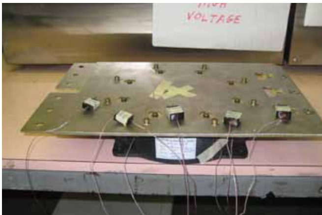
Figure 3: Photograph of instrumented 700D348 capacitor mounted on the bus plate assembly.
