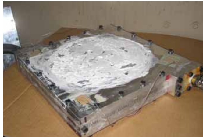
Figure 4: Heat transfer plate assembly showing thermocouples and thermal grease.
