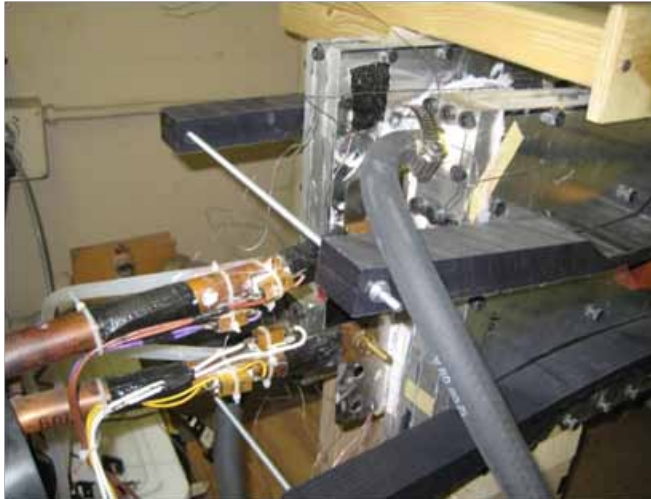
Figure 5: Capacitor assembly clamped between two heat transfer plates showing high current connections to the laminar bus assembly.
