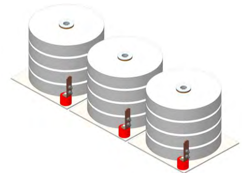
3-phase Horizontal Alignment
